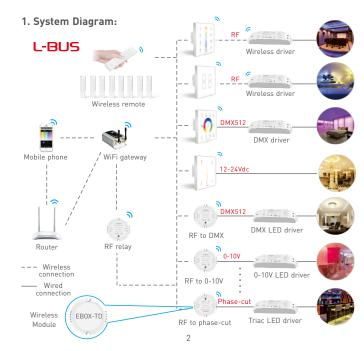
EBOX-TD wireless module applies L-BUS wireless communication protocol and converts it into trailing edge dimming signal through RF wireless communication technology, which is used together with LTECH Triac LED driver and compatible with all Triac series products in the market. Rely on L-BUS wireless technology application, it has removed the complex cabling procedure and expensive technical commissioning fee, to make it more easier for new or retrofit installations.
