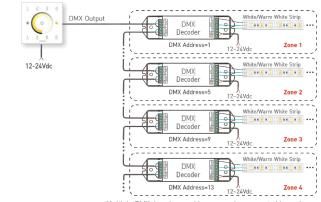
Multiple DMX decoders and lamps can be connected in each zone.
