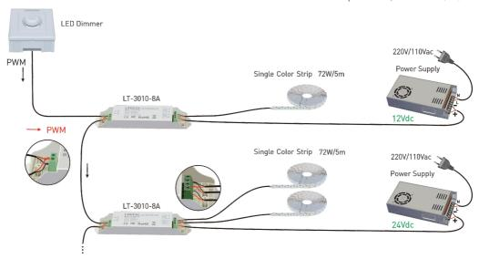
Power repeater connected to LED dimming driver:
