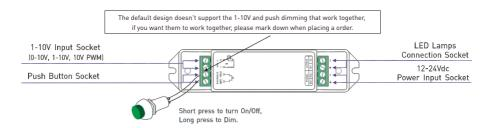
12V lamp connected, loads 0~72W(12V).
