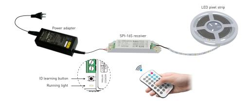
LED pixel strip wiring diagram:
