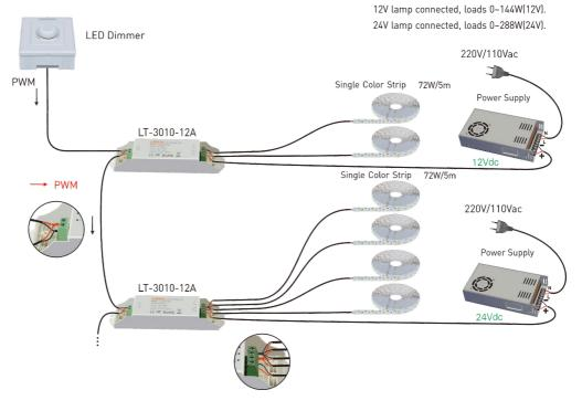
Power Repeater Connected to LED Dimmer:
