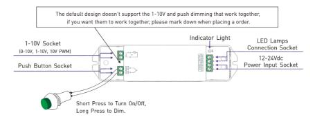
12V lamp connected, loads 0~144W(12V).
