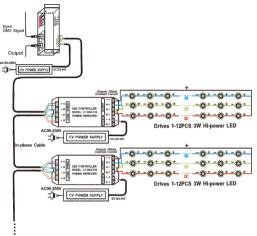
3. Repeaters Connected to LED Wall Dimmer as Follows:
