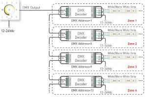
Multiple DMX decoders and lamps can be connected in each zone.
