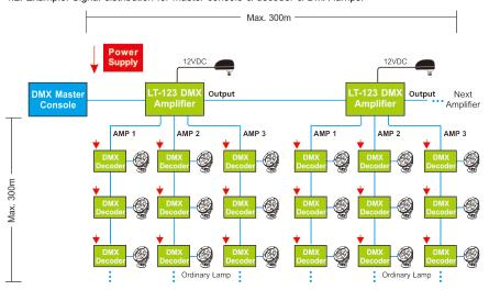
4.3 Example: Connection for signal amplifier in long distance:
